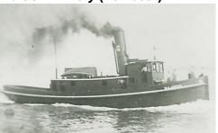
Built at Bay City, MI by P.W. Hitchcock & Co. in 1880.She was made of wood and was steam powered. Her measures were 78.8' x 16.8' x 7.9', with tonnage rated at: 70 grt 58 net. She was owned by W. H. Bridges, Bay City, Enrolled at Port Huron, June 10, 1880, she was assigned official number 80765.
