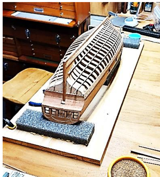
Hull, (above) with battens installed on port side.
