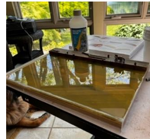
Once poured requires 42 hours to set up
