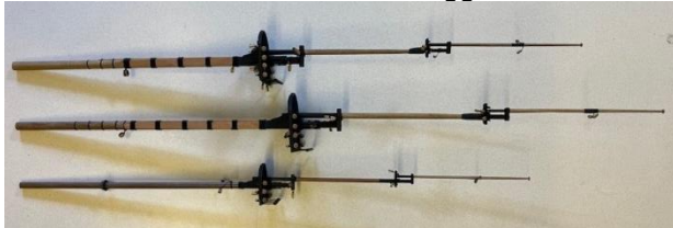
Masts built and sections painted black according to the plans. Blocks and other fittings were added.
