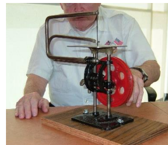
Loran brought is a 1923, hand-powered, scroll saw. Loen uses it rather than a powered scroll saw.
