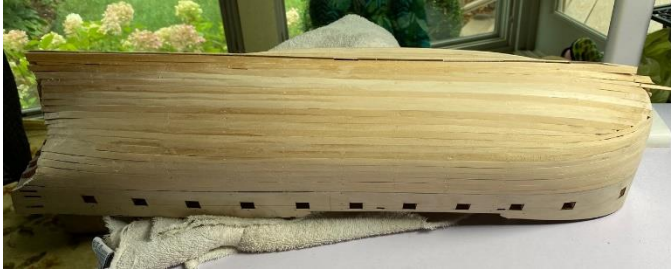
Second photo below, shows the second layer of Pear wood being applied:
