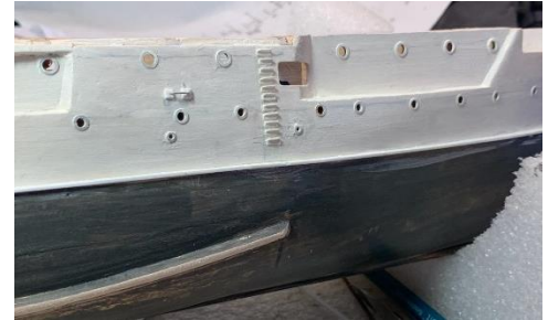
Above: Port holes & Haws Pipes
