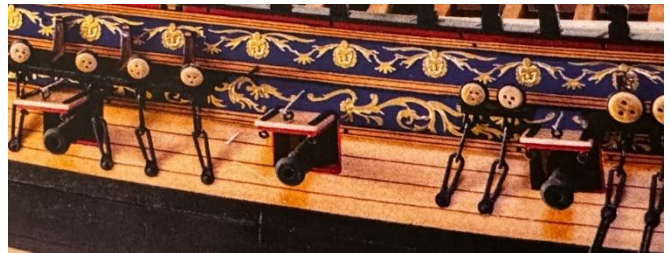
Gun Port Lids installed
