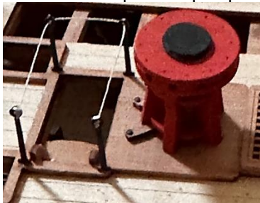
Ladder with ropes & top capstan
