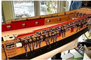
Cabin bulkheads installed along with windows
