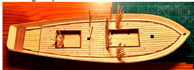
Julie is using toothpicks for treenail to fasten the deck to the frames. Nice work Julie.
