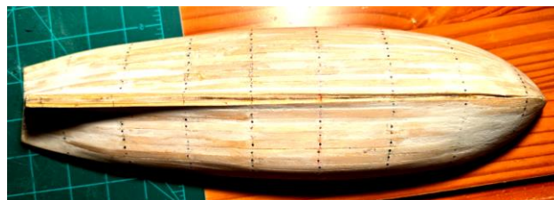
In the photo above, those are small brass nails fastening the planks to the frames.
