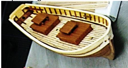
Completed planking of hull. Plans to add treenails.
