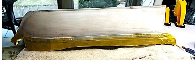
Ship is masked off and filler was used to make a good surface with no cracks or holes. Ronseal natural wood filler was used. Its advantage is that it can be watered down to a thin consistency.
