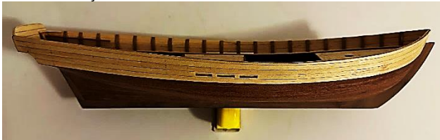
Completed planking of hull. Plans to add treenails.
