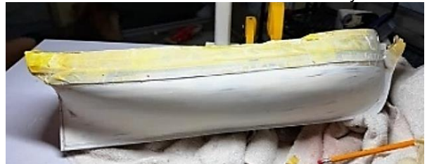
White primer airbrushed was then applied and will be followed by many coats of white acrylic paint. Each coat sanded until smooth.
