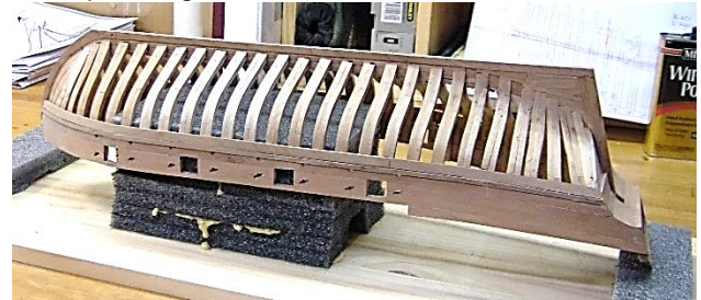
The second to hold the hull upside down while planking the hull below the waterline.
