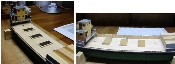
Above, the cargo hold deck showing hold comings and cargo hold lids. Need to add handholds to lids.
