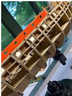
Completed gun deck bulkheads, installed the cabin floor and seat and fairing the sides in preparation for planking.
