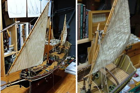
Sails cleaned, rigged and now dealing with how the attach the yards to the masts.
