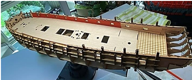
Completed gun deck bulkheads, installed the cabin floor and seat and fairing the sides in preparation for planking.
